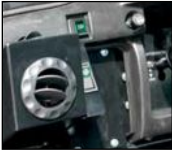
HEATER KIT With a two stage blower, this heater kit - which installs in the instrument panel - uses a heat exchanger to produce a warm atmosphere in your MULE cab when all around is cold.
