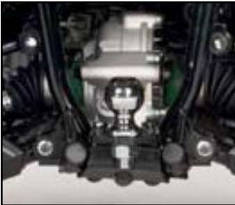
TOWBALL For many a towball is an essential accessory and this one is E-Approved for Europe. Ball = 50 mm diameter. Shaft = 24 mm, thread 20 mm diameter.
