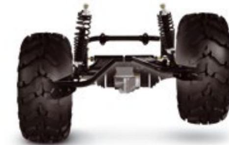
SUSPENSION ARRIERE INDEPENDANTE A BRAS TRIANGULAIRES D'ARTICULATION A TORSION (TTI)
