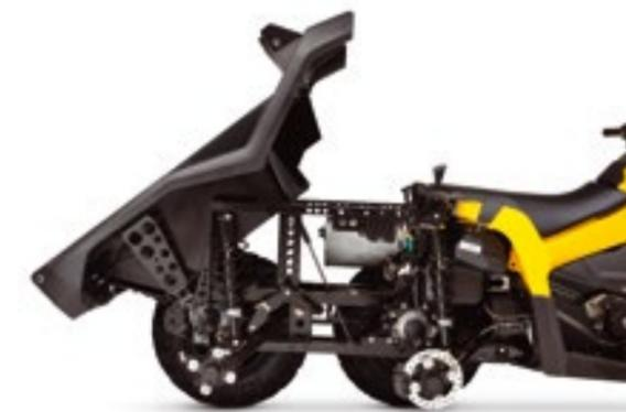
SUSPENSION ARRIERE INDEPENDANTE AVEC BRAS D'ARTICULATION A DOUBLE TORSION (TTI<sup>2</sup>)
