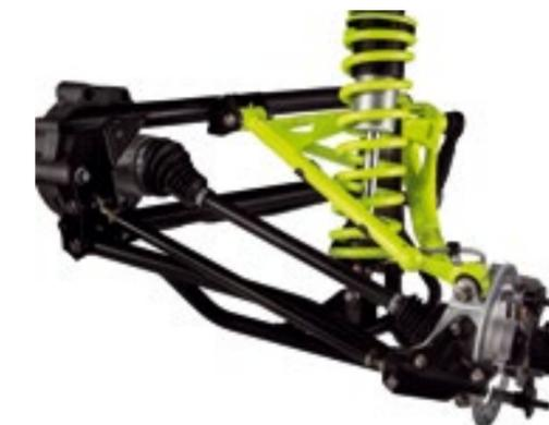
SUSPENSION ARRIERE AVEC BRAS TRIANGULAIRE D'ARTICULATION A TORSION (TTA)
